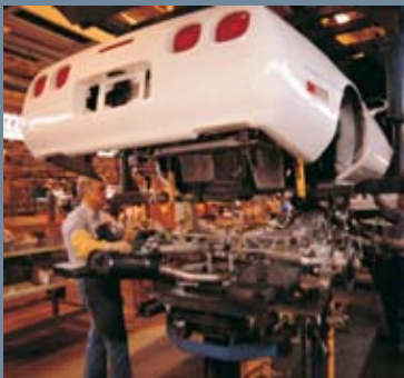
PosiTrack helps synchronize overhead and floor-based conveyors in chassis "marriage" systems.
